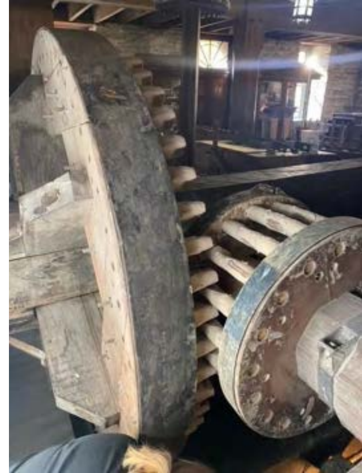
Interior side view of first gear to be replaced (wooden teeth replaced regularly)
